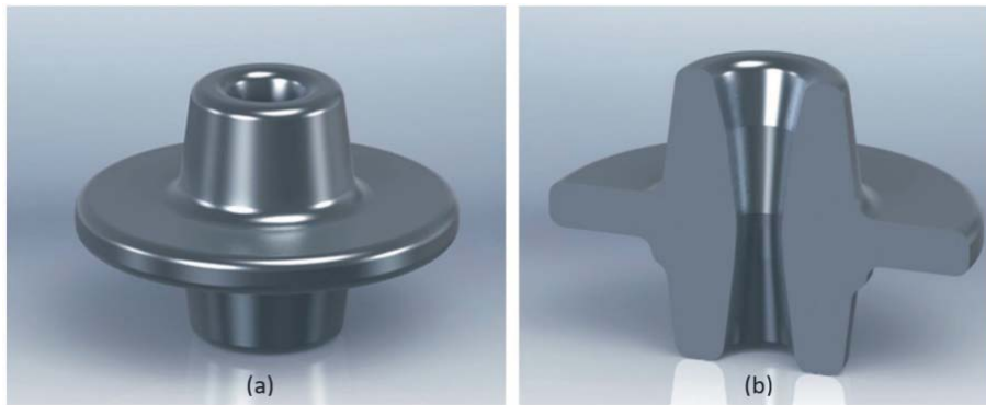
Fig. 2 (a) The 3D representation of the part to be forged; and (b) Cross-sectional view.
