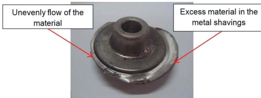
Fig. 12 First experiment: unevenly distributed of the material.
